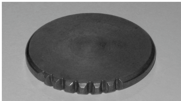
Coin, notched on one side to catch the wire firmly.
